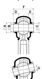
This protection completely conserves the rod-end bearing from any external attack:
