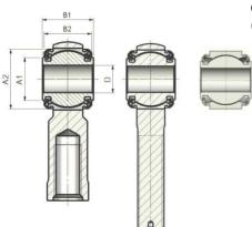
On request, we make sealed rod-end bearings, fitted with bellows. (minimum quantity required)
