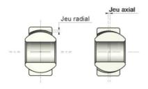
Spherical bearings and rod-end bearings have initial play or slip torque that is specific to the type and size.
