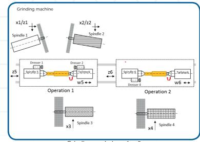
Grinding workpiece 2
